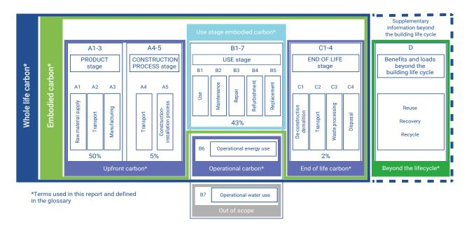
Figure 1: Life cycle stages and modules according to the Standard EN 15978 and the estimated distribution of emissions for a medium-scale residential building
